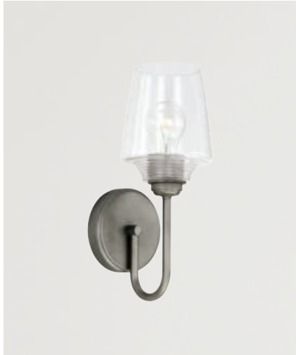
▲ 642211GR-512 SCONCE Graphite 642211AD-512 SCONCE Aged Brass 5.25"W x 13"H x 6.50"E Backplate: 5"W x 5"H x 1"E Ctr/Top: 4" Ctr/Btm: 9" 1 - 100 Watt E26 Medium Clear Ribbed Glass Damp Rated
